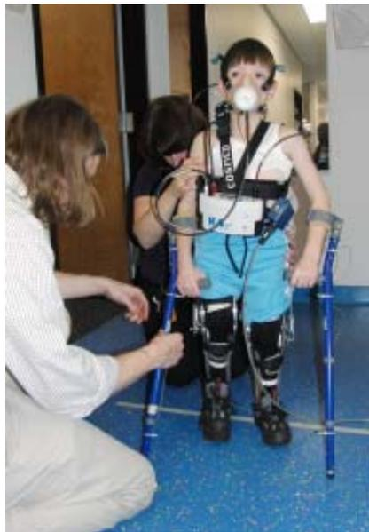
Figure 1: Subject wearing portable instrumentation for measuring gait.
