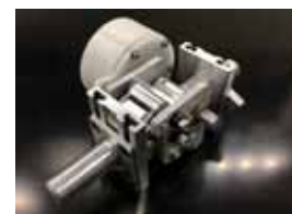
"Works-like" knee prototype with springs and dampers that engage at different times within the gait cycle.
