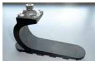
Prosthetic foot designed through LLTE optimization. Can be injection molded for under $10 USD.
