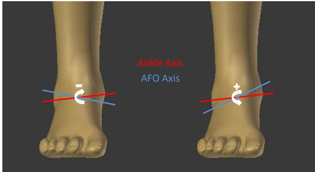
The AFO axis can be rotated relative to the anatomical ankle axis in the coronal plane. Once again, rotations in the frontal plane only affect the orientation of the AFO axis relative to the ankle axis, not its position. The above image indicates the sign associated with each rotation direction.
